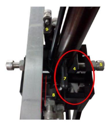
It may also be seen in the image above that the adjustment of the side backstop is incorrect, because axle 7 is not engaged to part 8.
