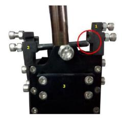
This problem may be caused by an incorrect adjustment of part 3. It is not recommended to change the original height of this part under any circumstances. Observe in the picture below where the height of part 3 was changed.
