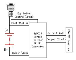
The voltage of the Key switch control is consistent with the input voltage
